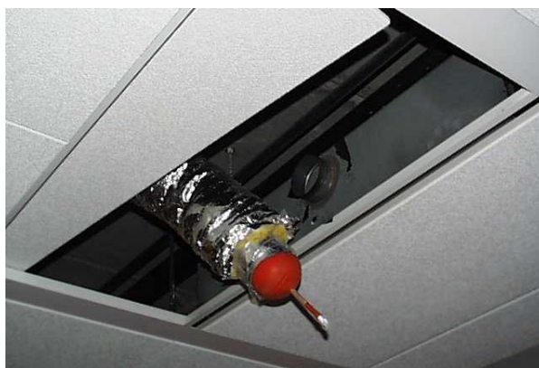
Figure 52: Measurement with disconnected plenum (in this case plenum for linear register)
