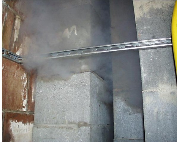
Figure 53: Smoke visualisation of leaks in a concrete ductwork.
