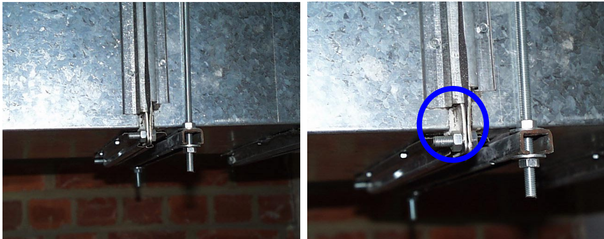
Figure 23: Detail of a leak during and at the end of the test. The white material indicated by the circle on the right hand-side is the seal created by the deposition of aerosol particles.
