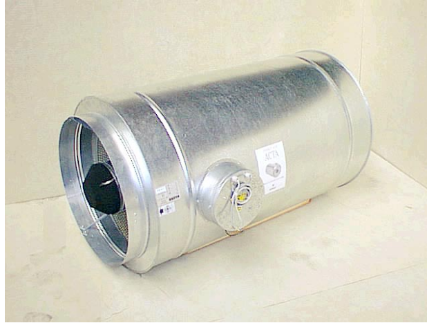
Figure 5: Cylindrical type silencer combining passive sound attenuation by rock wool with reactive attenuation (neutralisation of noise by the addition of opposite sound). The Noise Negator is used as a component in the HVAC systems of commercial buildings or domestic dwellings (courtesy ALDES Aéraulique).
